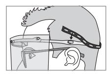
For extra stability, attach the buttonhole elastic strap to the rear mounts of the visor carrier and adjust it as required.
