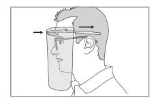
Put on the face shield by holding the temples of the visor carrier at forehead height and sliding them horizontally towards the back of the head. Spectacle wearers can also place the carrier on the frame of their glasses.
