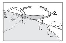
First, press the two centre holes of the visor foil onto the mounts on the visor carrier. Continue with the two outer holes. Your face shield is now ready for use.
