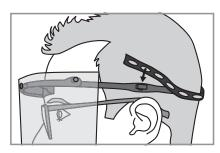
For extra stability, attach the buttonhole elastic strap to the rear mounts of the visor carrier and adjust it as required.
