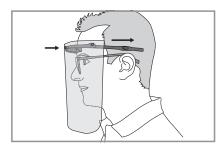
Put on the face shield by holding the temples of the visor carrier at forehead height and sliding them horizontally towards the back of the head. Spectacle wearers can also place the carrier on the frame of their glasses.
