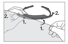
First, press the two centre holes of the foil onto the mounts on the visor carrier. Continue with the two outer holes. Your face shield is now ready for use.
